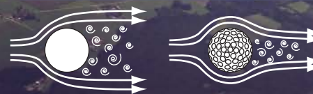
a) Golfball without dimples: Strong boundary layer separation b) Golfball with dimples: lower boundary layer separation
